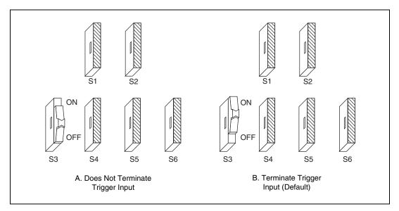
Figure C-7. SMB Trigger Input Termination
